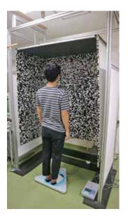
**Figure 1** Experimental design. A participant stands in a box, the inside of which was randomly dotted and is instructed to look at the randomly dotted pattern. The box suddenly begins to swing, approaching the participant, and continues to swing back and forth in a damped sinusoidal waveform. Body center sway was recorded using a stabilometer.
